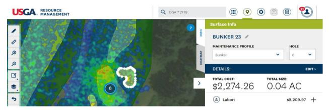
As noted in the screenshot, a large portion of this bunker can be eliminated to reduce the cost of annual maintenance by over \$1,350. Also, note that the major expense involved with bunker maintenance is the labor portion. Very little gasoline and other materials are used for bunker maintenance, however when new sand is added this will increase overall costs. By downsizing or removing bunkers, all of this labor will be used for in-play areas to enhance playing conditions.
